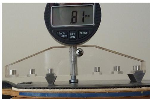
**4. Racket Covering Thickness Test**
